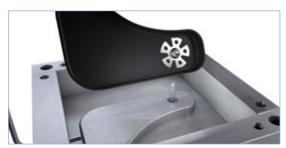
The assembly is removed from the mould.
