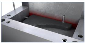
The mould closes over the system to be assembled, so as to ensure perfect sealing. An epoxy resin is then injected and cured. The composite is hardened, and the insert is then moulded-in.
