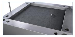
The preimpregnated material is introduced in the mould. The fibres remain continuous.
